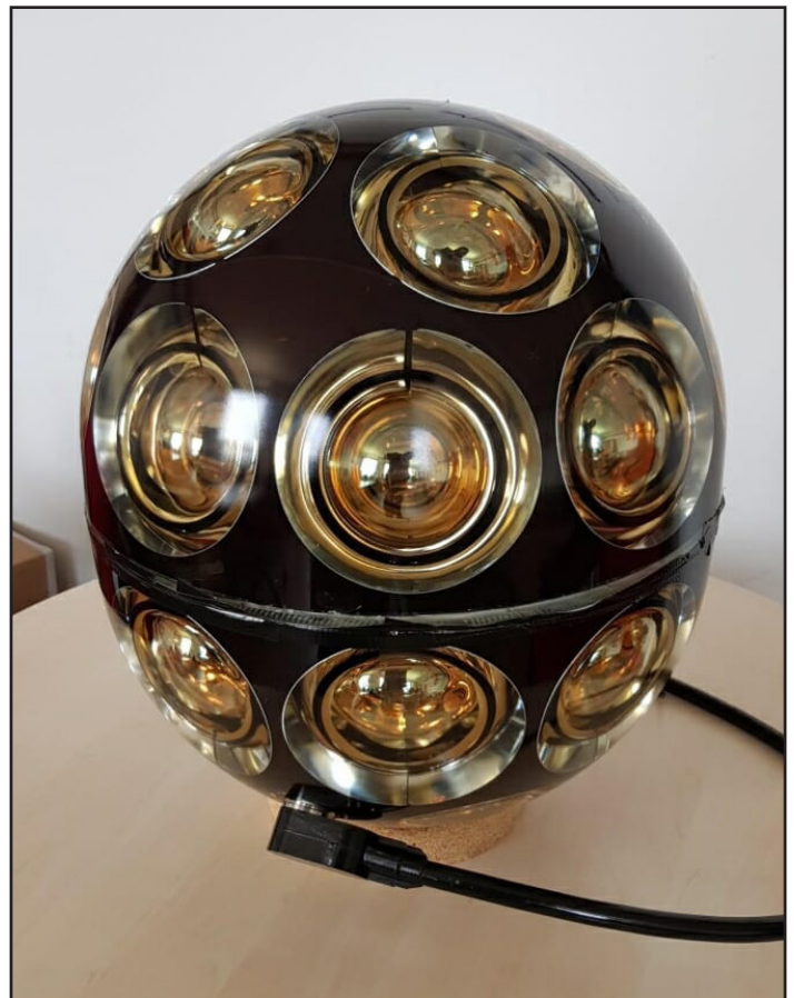
A prototype of one of the IceCube Upgrade project's new sensor module designs, called the mDOM, which has multiple photomultiplier tubes arranged for uniform sensitivity.
