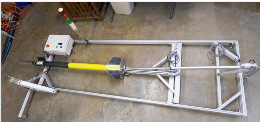
Top view of completed Automated Ground Support Equipment (AGSE) with sample return rocket Mars Ascent Vehicle (MAV). This winning design weighed only 86 pounds and had a volume of less than 9 by 2.5 by 1.5 feet overall, and accomplished the task of loading and securing the payload and erecting the rocket for launch in less than 55 seconds.
