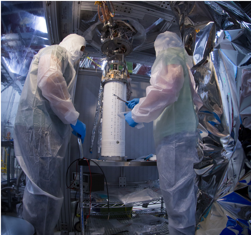
Scientists from the LZ collaboration install the system test prototype detector for its first run at the SLAC National Accelerator Laboratory.
