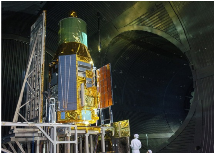
Completed spacecraft in the thermal-vacuum test chamber
