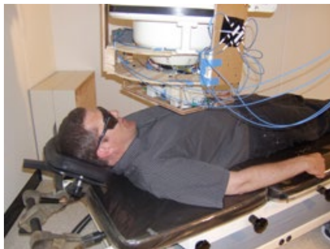
Photo: Professor Walker getting his magneto-cardiogram measured by the UW ultrasensitive magnetometer array.
