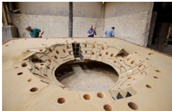
Figure: On June 16, 2011, workers at Portage Casting and Mold Inc. in Portage, Wis., assembled a five-section-mold needed for the main vacuum vessel of the Plasma Dynamo Facility at UW-Madison.
