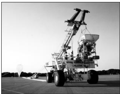
Our telescope gondola on the launch pad, ready for a balloon flight to observe the 2.7 K cosmic microwave background radiation. A scientific helium balloon is filling in the background. The truck (“Tiny Tim”) holds the gondola until launch.
