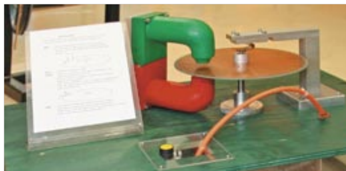
Dynamo demonstrating a force exerted by a magnetic field on an electrical current.
