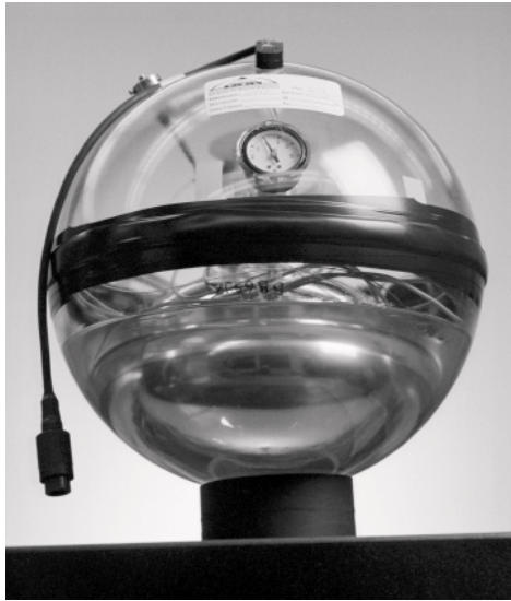
The photomultiplier tubes within these basketball-sized glass orbs are at the heart of the AMANDA neutrino telescope, a novel telescope being built at the South Pole to detect cosmic neutrinos.
