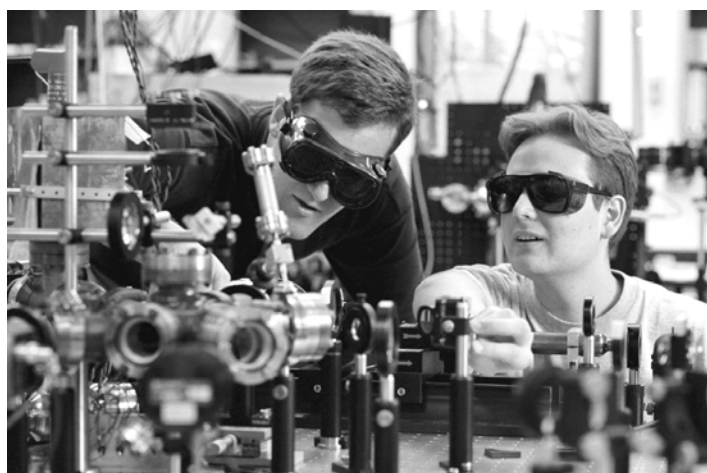
"Physicist Thad Walker, left, and senior Nathan Harrison, right, adjust infrared laser equipment used to trap and cool atoms to near absolute zero. By using a special infrared lens, one can see a tiny green ball of light, smaller than a marble, that constitutes the trapped atoms scattering laser light. It can take more than a year to set up a functional atom trap." Photo: Jeff Miller
